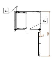
**Electric** Supply voltage: 220-240 V/1 ph/50 Hz Electrical power, max: 0.45 kW Capacity: Number and type of grids (included): 5 - 530x700 **Key Information:** Net Volume: 510 It
